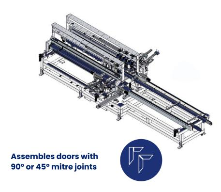
The machine can be equipped with either a fully automatic or semi-automatic feeding depending on requirements in terms of production and flexibility.
